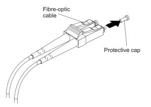
Figure 31. Removing fiber-optic cable protective caps
